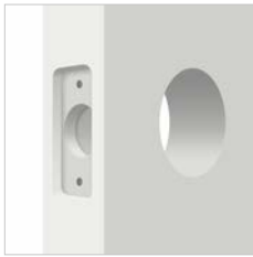
LOCK preparation for standard doorknob with 2 3/8" backset
